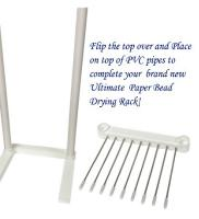
**Step 3:** Insert the two 15" long PVC pipes into the base. This photo shows the base partially assembled, what is left
